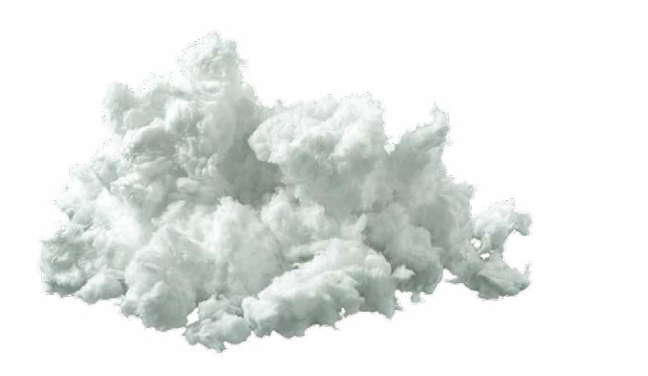
Example of blown in Glasswool
