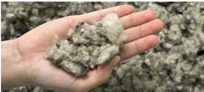
Example of blown in Rockwool
