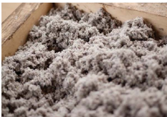
Examples of blown in Cellulose fibre
